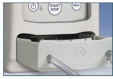
2. Insert disposable cassette tubing into cartridge slot, by placing thumb on the "arrow" & fingers on the grasping handle located at the bottom of the pump.
