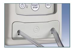
3. Press tubing cassette into FloSteady pump until it "snaps" in. The cassette tubing is now inserted and ready to use.
